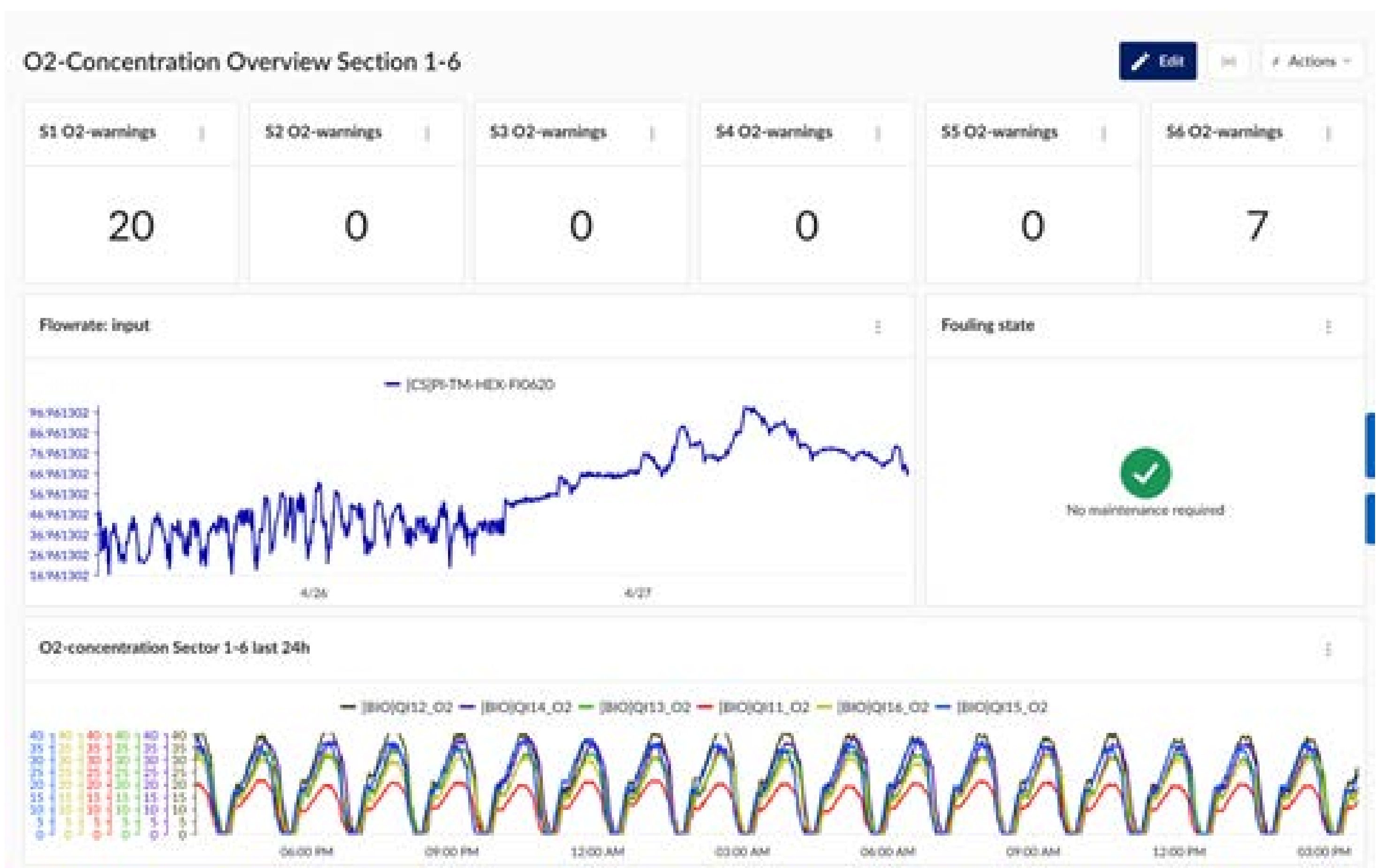
Figure 11. Maintenance Dashboard to monitor the fouling state of aeration elements.
